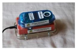
SI Master on top of Master Station connected by black magnetic stick
