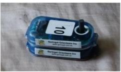
Control 10 on top of Master Station connected by black magnetic stick
